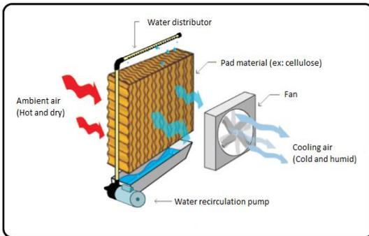
Figure 1. EAC at UFGD laboratories and operating sketch from manufacturer.
