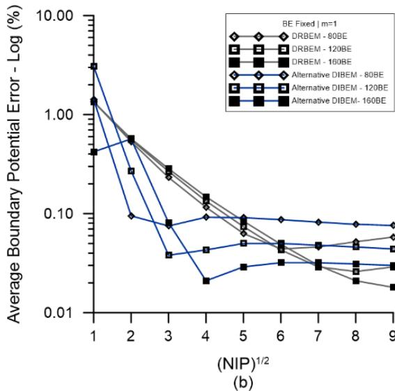
Figure 3- Convergence Analysis: (a) Classical DIBEM vs. Alternative DIBEM (b) Alternative DIBEM vs. DRBEM
