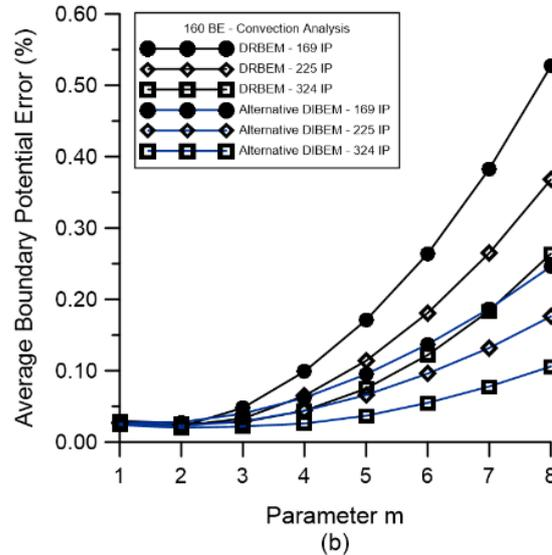
Figure 4- Parametric Analysis with m: (a) Classical DIBEM vs. Alternative DIBEM (b) Alternative DIBEM vs. DRBEM
