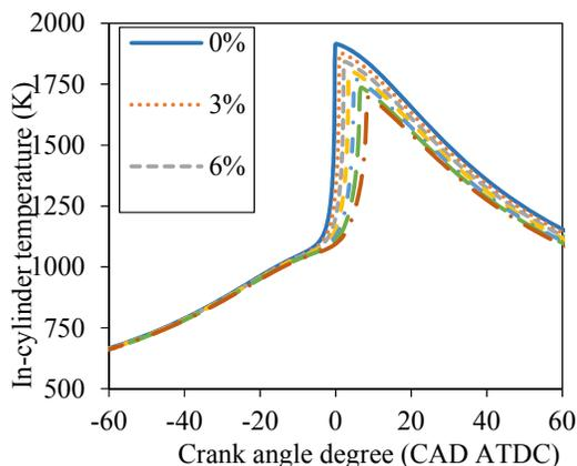
Figure 4 - In-cylinder temperature in relation to water fraction (% in mass basis)
