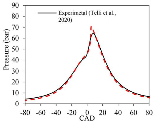
Figure 1 - Comparison of the present numerical model with experimental data from Telli *et al.*, (2020). CR = 14:1, N = 1800 rpm,  $T_{in}$  = 406 K,  $P_{in}$  = 1.4 bar, and  $\lambda$  = 1.4, H<sub>2</sub>O injected = 7% mass basis.
