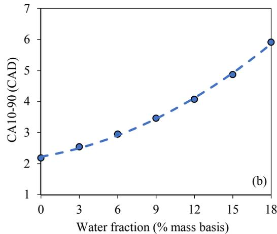
Figure 5 – Start of combustion, CA50 (a) and CA10 90 (b) in relation to water fraction (% in mass basis)
