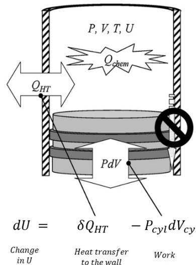
Figure 1 - Scheme of the first law of thermodynamics for single-zone models (Konninos and Rakopoulos, 2012)
