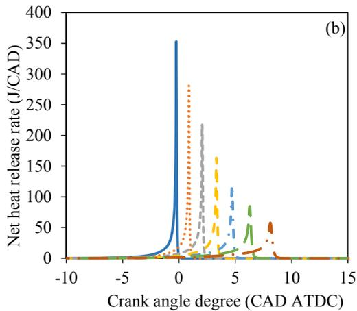
Figure 3 – In-cylinder pressure (a) and net heat release rate (b) in relation to water fraction (% in mass basis)
