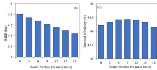
Figure 6 – IMEP and thermal efficiency in relation to water fraction (% in mass basis)
