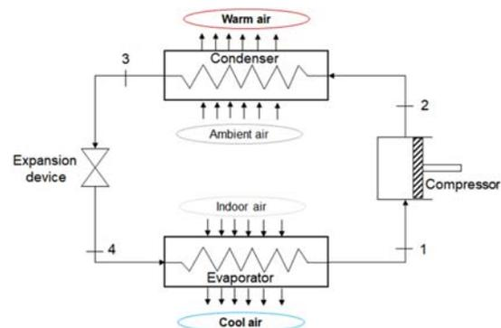
Figure 1. Vapor compression refrigeration cycle for an air conditioning.
