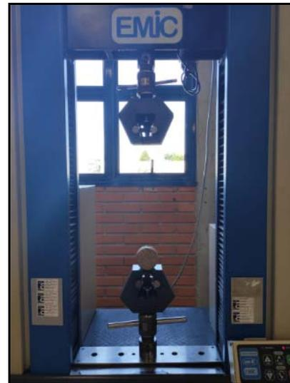
Figure 4. Diametrical compressive strength test equipment.
