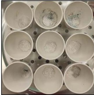
Figure 10. Ash Content of samples.
