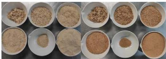
Figure 7. Particle size distribution of pine and cambará sawdust, respectively.
