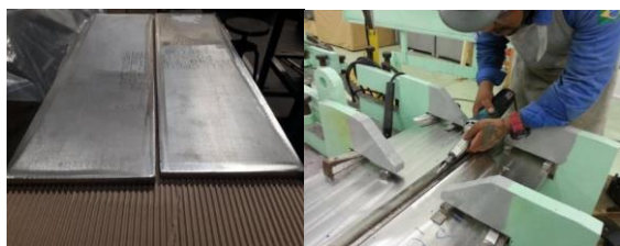
Figure 3. Cutting of Sample Sheets and Preparation for Welding.
