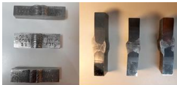
Figure 10 - Macrograph of samples A-B C-D and E-F, respectively
