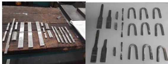
Figure 8 - Machining of specimens, specimens of traction and folding
