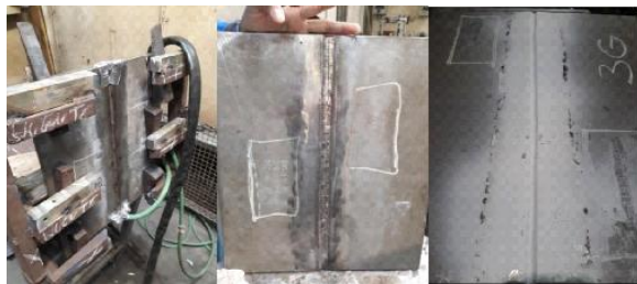
Figure 4. Welding of samples used for the removal of specimens of WPQ.
