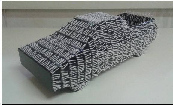
Figure 6. Pickup model with wool tufts.
