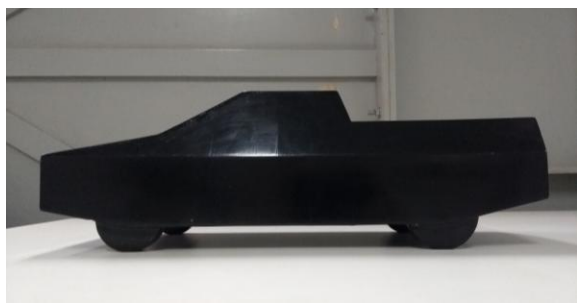
Figure 3. Pickup truck test article ( 1/10^{\text{th}} scale).
