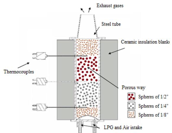
Figure 3. Porous matrix distribution adapted from REGO, 2016.
