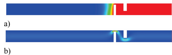
Figure 11. a) Temperature field for Be = 1.828 and H_3/L_3 = 4.0 , b) Velocity field for Be = 1.828 and H_3/L_3 = 4.0 .
