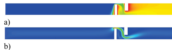
Figure 12. a) Temperature field for Re_H = 100 and H_3/L_3 = 4.0 , b) Velocity field for Re_H = 100 and H_3/L_3 = 4.0 .
