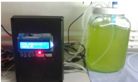
Figure 3. Automated Photobioreactor used in experiments.
