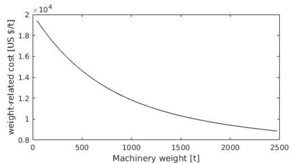
Figure 6. Approximate costs of machinery per tonne.
