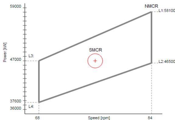
Figure 5. Engine layout diagram of the engine
