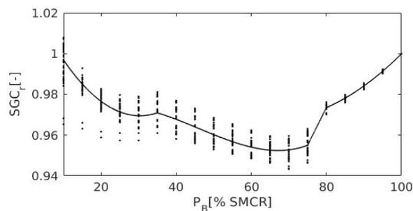
Figure 8. Fitted curve of relative specific gas consumption.
