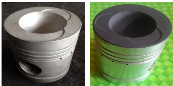
Figure 3. Pistons before and after coating with \text{TiO}_2 powder.
