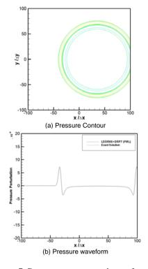
Figure 7. Pressure contours and waveforms – LDDRK5+DRP7, M=0.5, CFL = 0.1.
