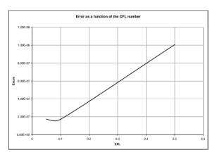
Figure 4. Residual error vs CFL number – Case (A) problem. LDDRK5+DRP7 (outflow boundary condition applied).
