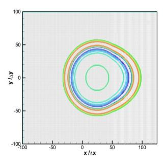
Figure 11 – Effect of grid stretching over the acoustic pulse propagation – LDDRK5+DRP7, M=0.5, CFL = 0.1. Pressure contours.
