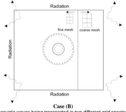
Acoustic waves being transported in two different grid spacing;
