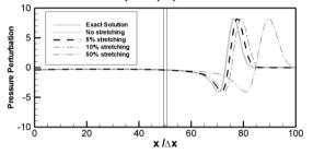
Figure 10. Effect of grid stretching over the acoustic pulse propagation – LDDRK5+DRP7, M=0.5, CFL = 0.1. The interface between the two mesh resolutions is marked with double-line.
