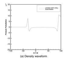
Figure 8. Density waveform – LDDRK5+DRP7, M=0.5, CFL = 0.1.
