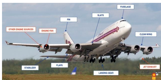
Figure 1. Aircraft and noise sources.
