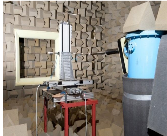
Figure 5. General view of Doak Laboratory with traverse system to hot-wire anemometer and Pitot tube measurements.
