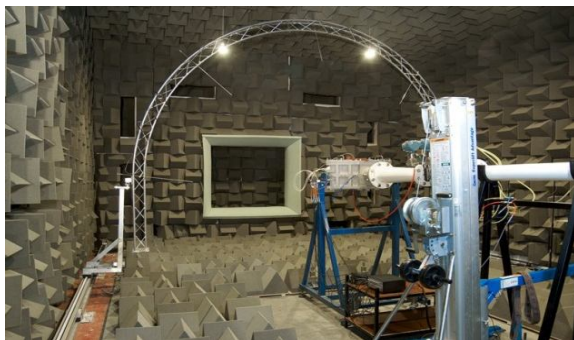
Figure 3. Anechoic chamber at DOAK Laboratory during antransversable azimuthal array of microphones experiment.
