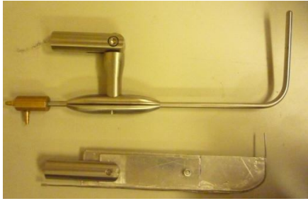
Figure 6. Pitot tube of the micromanometer and Pitot tube built during the experiments by Mat Gruber.
