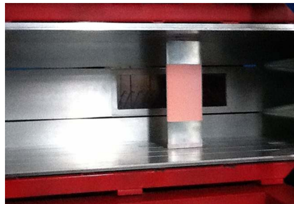
Figure 5. NACA0012 profile in the wind tunnel test section.
