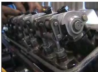
Figure 4. Rocker arm mounted in the motor.
