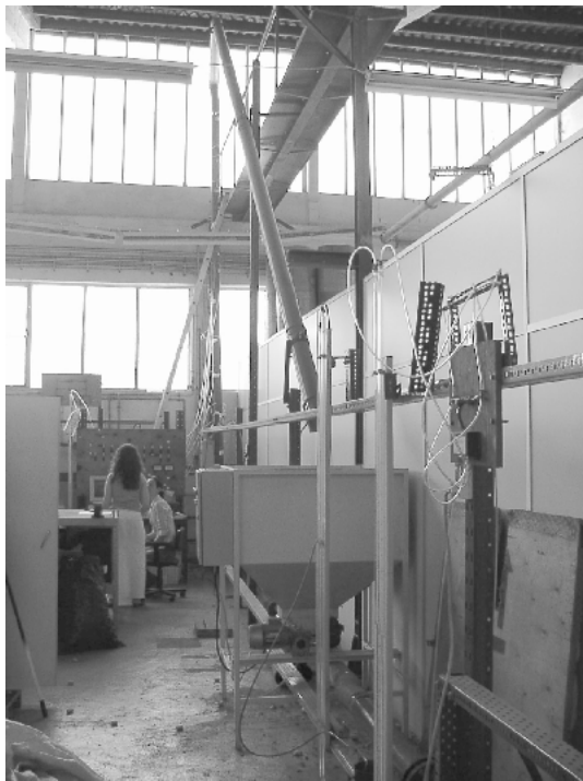
Figure 2. Experimental installation. In the first plan it can be seen the orifice plate air flow meter and the corks feeding hopper.
