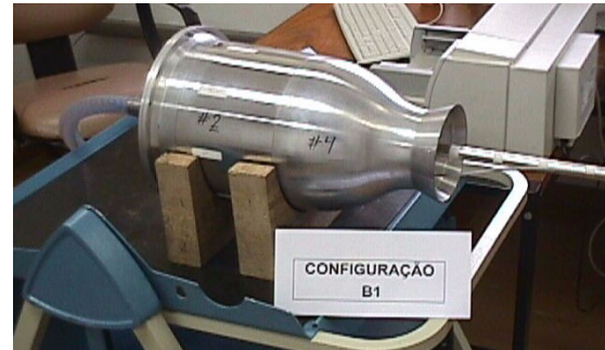
Figure 4. Position of acoustic liner along combustion chamber.
