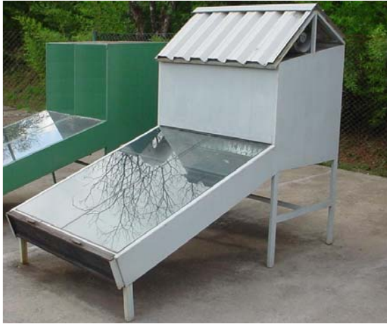
Figure 1. Hybrid solar-electrical dryer
