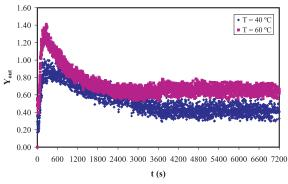
Figure 3. Drying air humidity curves in the dryer outlet.
