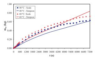
Figure 4. Comparison of the accumulated loss curves of water from analytical scale and from psychrometry (Simpson's rule).
