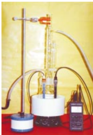
Fig. 1 - Equipment developed for immersion tests.
