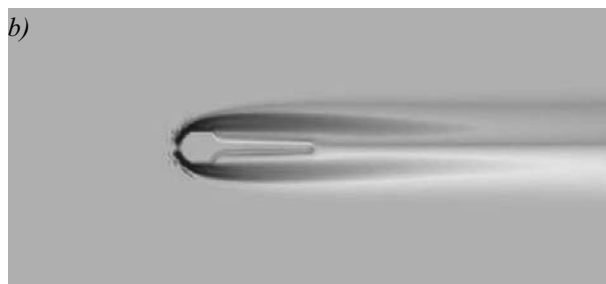
Figure 3. Vorticity field for Re = 100 at time t \cdot U_{\infty}/D = 347 ; a) l/D = 2 , b) l/D = 3 .
