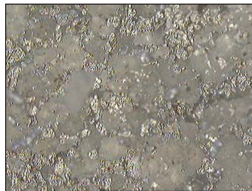
Figure 4. 70%Al/30% MDPE mixture after simultaneous compacting and heating at 200°C
