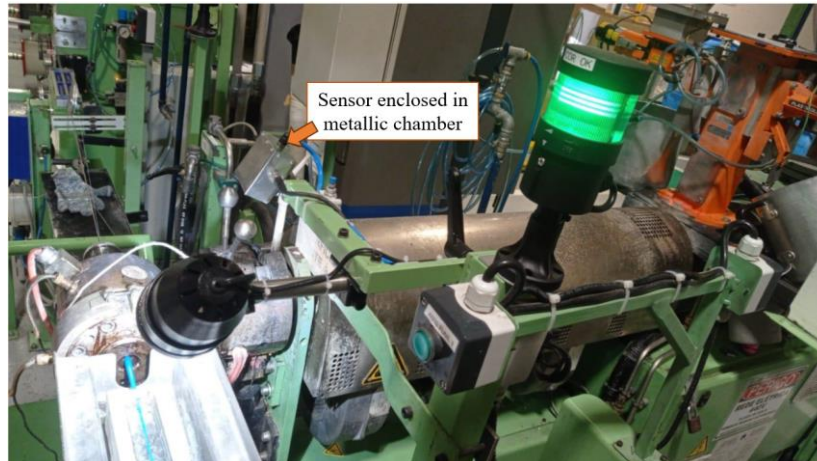
FIGURE 6. LIGHT SIGNAL INDICATING THE COLOR CONFORMITY OF A BLUE TUBE IN PRODUCTION
