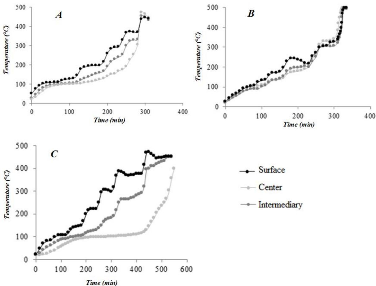
**Figure 2** - Graphical representation of the thermal gradient formed in wood A, B and C samples during slow pyrolysis.
