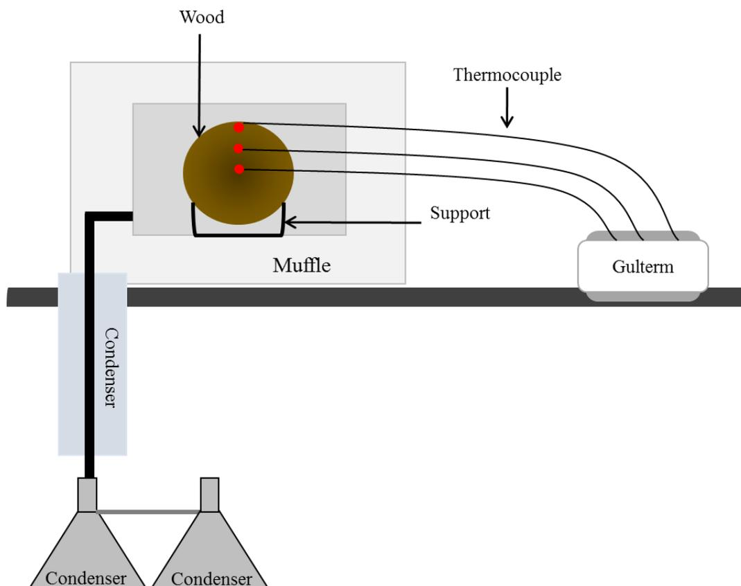
**Figure 1** - Layout of the carbonization system used in the experiments.
