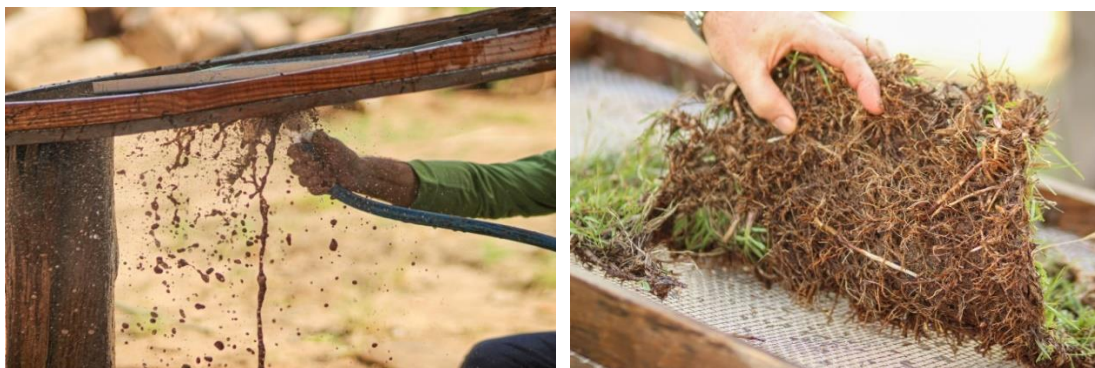
Figure 2 - Demonstration of the washing process of the samples for the soil removal in them. (Source: Authors, 2022).
