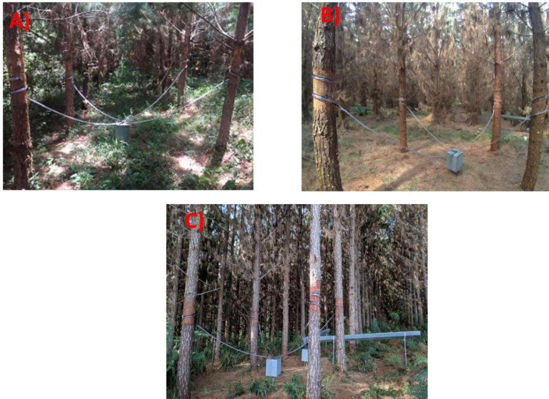
Figure 3 - Images of the three experiments and their respective stemflow collection systems, throughfall collection troughs, and tipping bucket shelters. A) E1 (5-year-old plantation), B) E2 (7-year-old plantation) and C) E3 (10-year-old plantation). Authors' production (2024).
