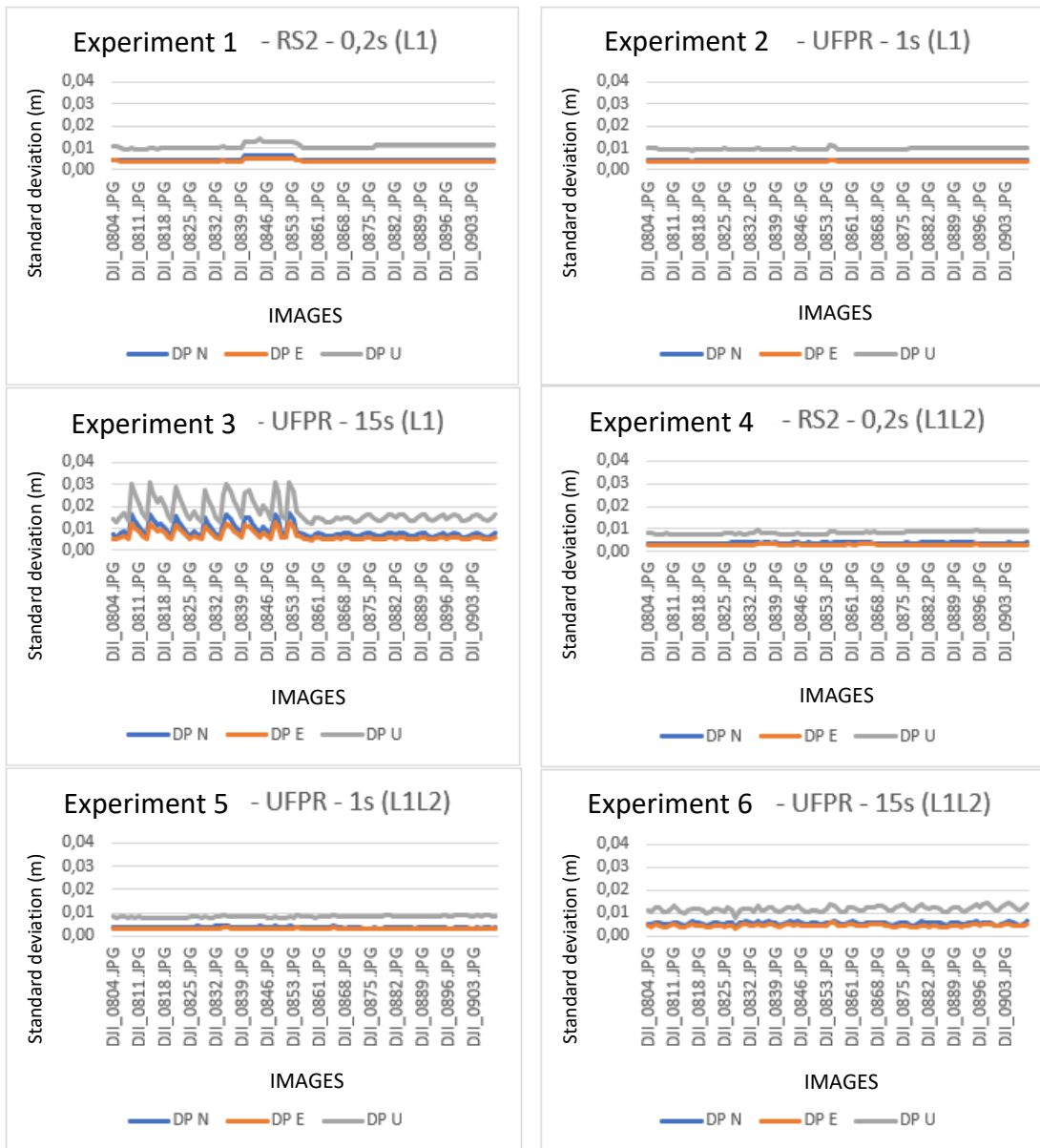
Figure 5 – Coordinate accuracies E, N and U of CP for experiments 1 to 6 with short LB. (prepared by the authors).
