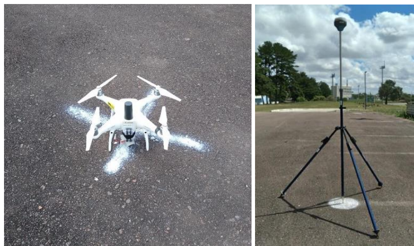
Figure 3 – DJI PHANTOM 4 ADVANCED, with the Guandalini PPK2 KIT attached and an example of field tracking with a marked point. (prepared by authors).
