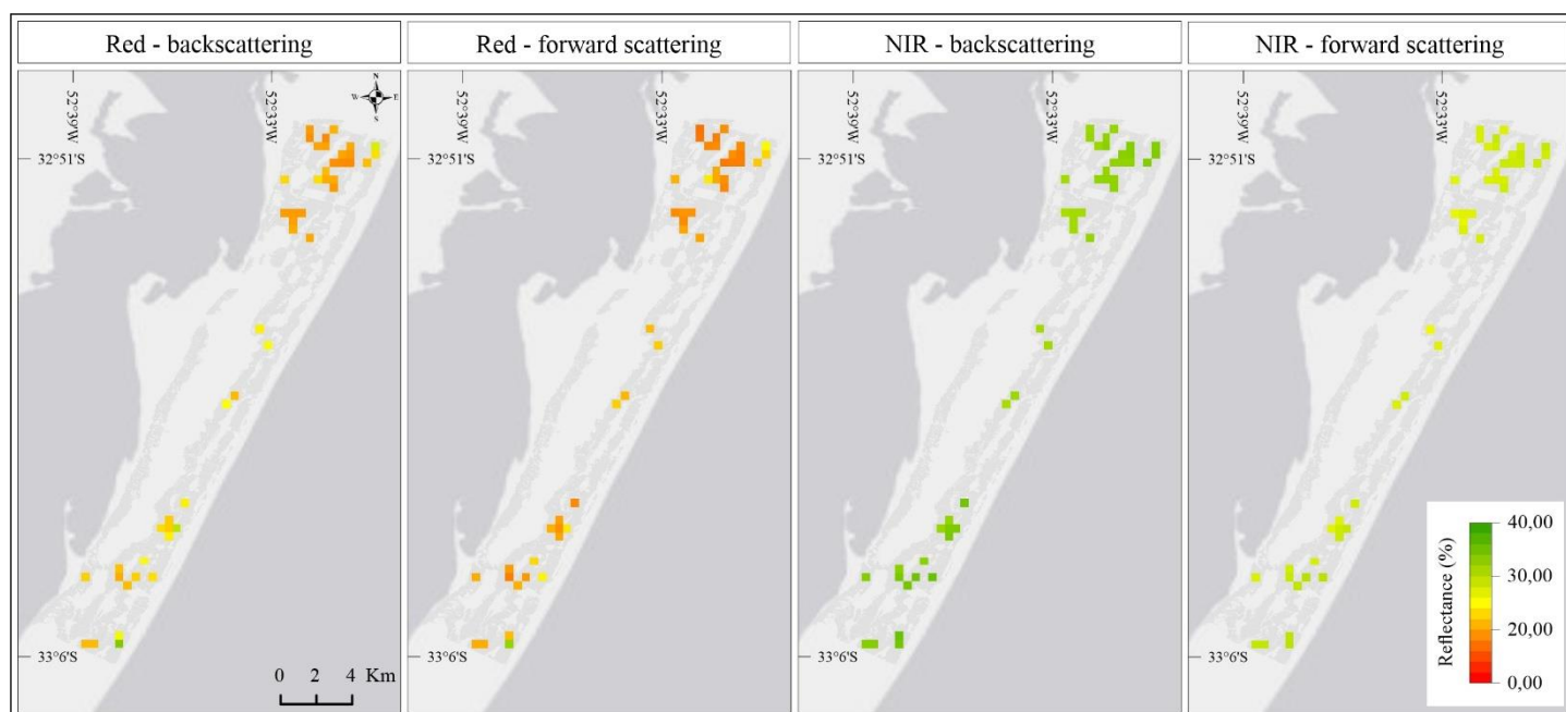
Figure 4 – Spatial variation of mean reflectance values from the multitemporal series of canopy observations, obtained from backscattering and forward scattering directions, for the red and near-infrared bands of the MODIS sensor. Source: prepared with data from the MOD09GA product (VERMOTE; WOLFE, 2015).
