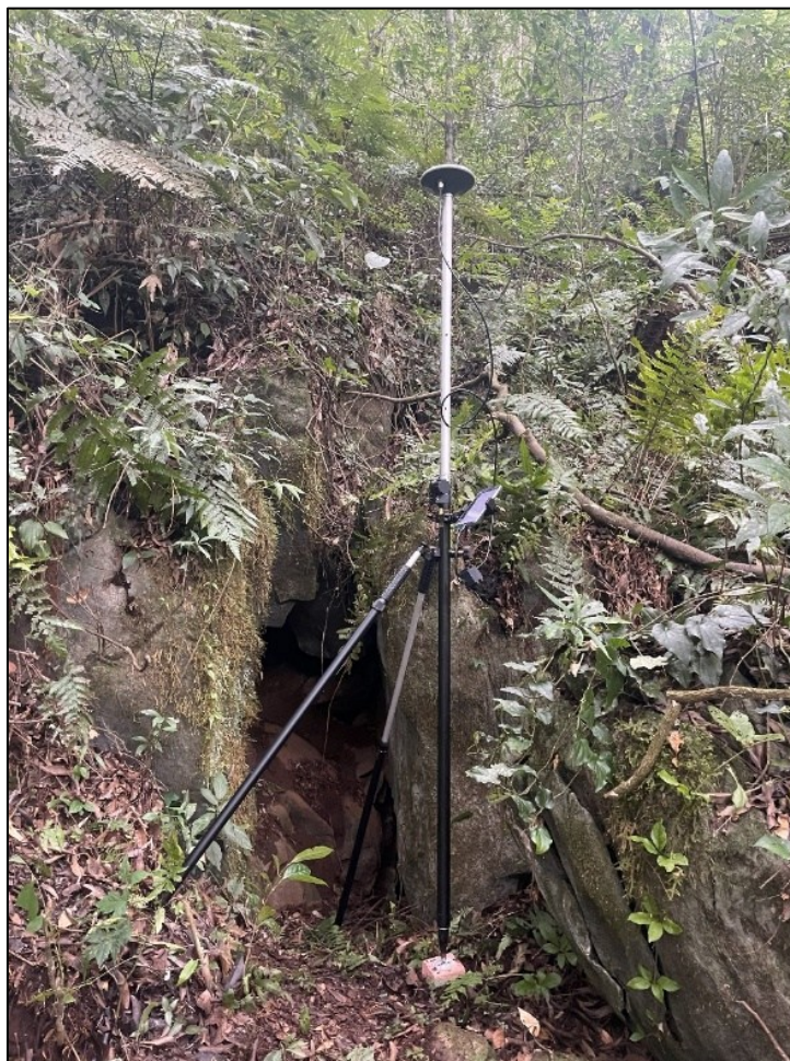
Figure 2 – Receiver system installed on a topographic benchmark for GNSS signal tracking (Gruta Taici I) and determination of coordinates (latitude and longitude) and elevation.
