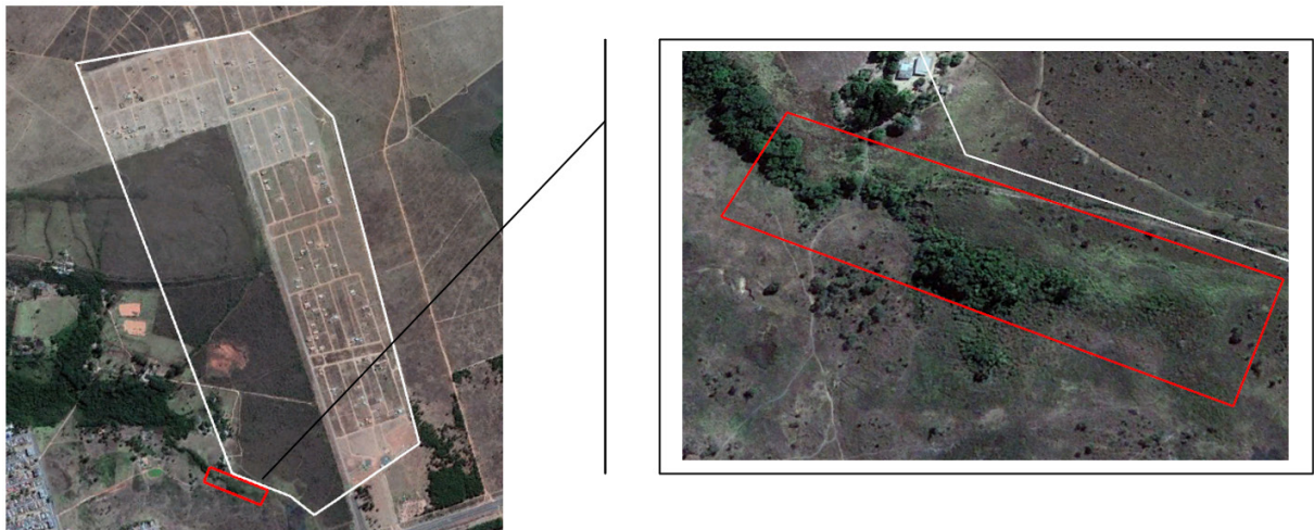
FIGURE 10 - The area recorded in the red rectangle in 2004 does not show a gully, which appears in 2015. SOURCE: Produced by the Authors, based on Google Earth (2022).
