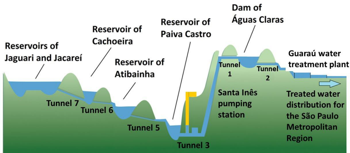
FIGURE 2 – Schematic diagram of the Cantareira System.
