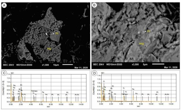
**Figure** - (A) Platinum crystal (Pt) included in a magnetite crystal (mg); (B) platinum (Pt) microcrystal in titanomagnetite (tmg) crystal; (C) EDS spectrum on the platinum microcrystal seen in Figure A; (D) EDS spectrum on the Pt microcrystal in the titanomagnetite crystal seen in Figure B.
