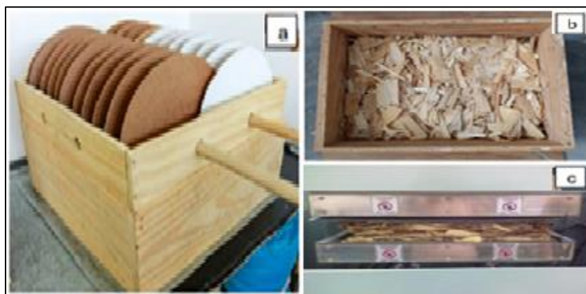
Figure 1. Panel manufacturing process, where (a) Wood Aligner built for the laboratory; (b) oriented particle mattress; (c) pressing.
