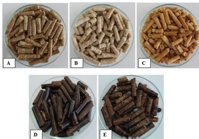
Figure 2. Pellets produced from raw and torrefied biomass.
