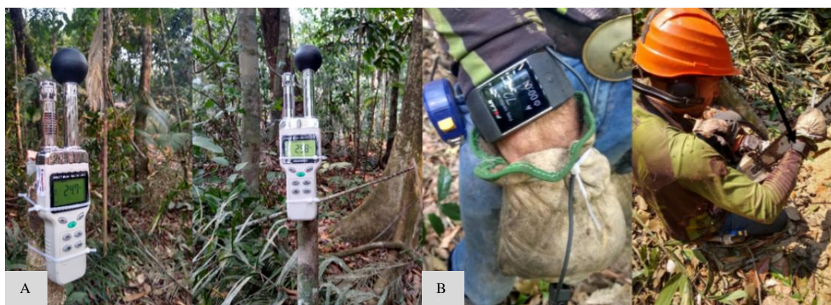
Figure 2. A: IBUTG portable digital thermometer installed on the banks of the storage yard. B: Heart rate meter installed on the chainsaw operator's wrist.
