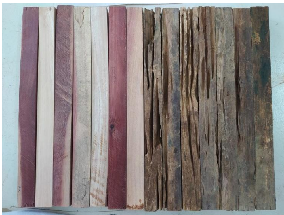
Figure 1. Woods of M. urundeuva before and after exposure to the soil.
