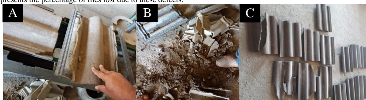
Figure 1. Adhesion to form (A), disaggregation (B), and breakage of the tiles (C).
