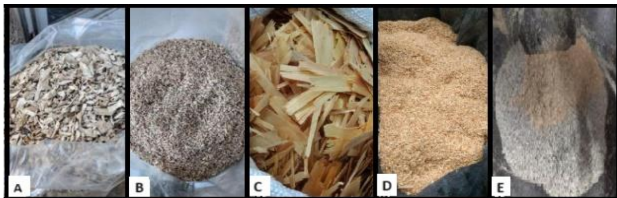
Figure 1. Production of particles to produce MDP panels. (A) Wood chip of Ilex paraguariensis ; (B) Sliver-type particles of Ilex paraguariensis wood; (C) Strand-type particle of Pinus taeda wood; (D) Sliver-type particle of Pinus taeda wood; (E) Sliver-type particles before being mixed in the proportion 60% Ilex paraguariensis /40% Pinus taeda .
