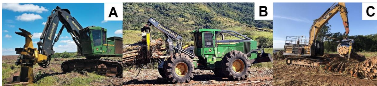
Figura 1. (A) Feller buncher , fabricante John Deere , modelo 903M; (B) Grapple skidder , fabricante John Deere , modelo 848H; (C) Grapple saw , fabricante Caterpillar , modelo 336D2L.
