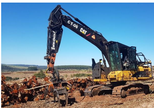
Figure 1. Self-propelled forestry machine grapple saw.
