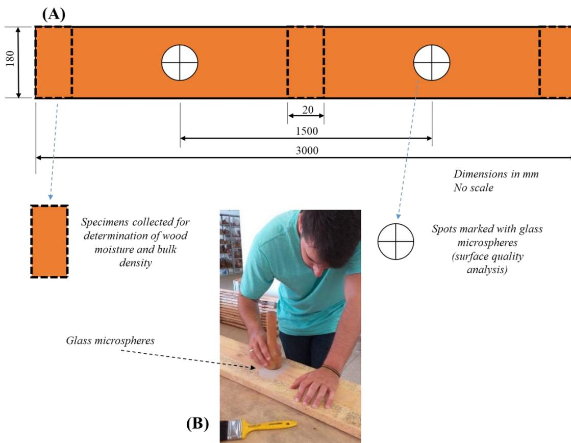
Figure 2. (A) Points used for surface quality assessment and specimen collection for determination of bulk density and moisture in boards of *Pinus caribaea* var. *caribaea* and (B) application of glass microspheres to the board surface.
