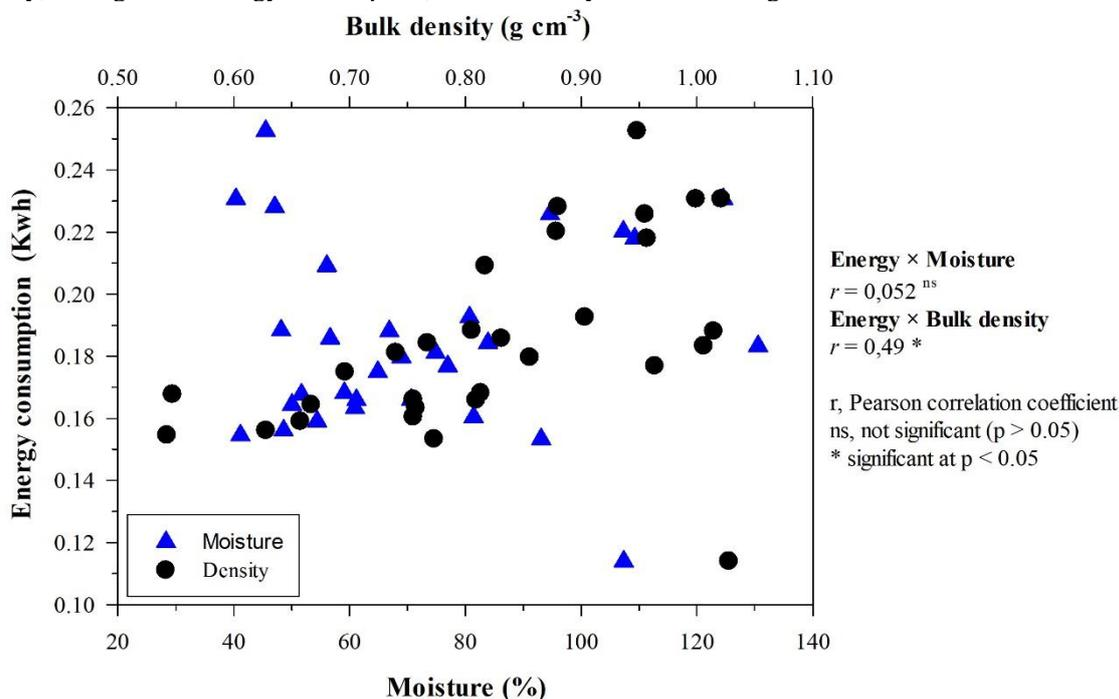
Figure 4. Scatterplot of portable sawmill energy consumption and the moisture and bulk density of *Pinus caribaea* var. *caribaea* lumber.
