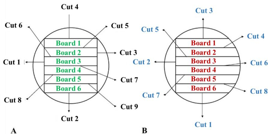
Figure 1. Breakdown of *Pinus caribaea* var. *caribaea* logs on a portable sawmill. Cutting sequences and board positions of (A) cant and (B) two-sided cant sawing patterns.
