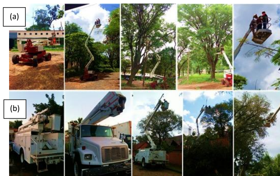
Figure 1. Articulated boom lift (a) and truck mounted boom lift (b) used in urban tree pruning operation.
