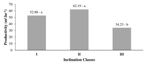
Averages followed by the same letters do not differ statistically between themselves by Tukey test at 5% level (p > 0,05). Figura 2. Produtividade média ( $m^3 he^{-1}$ ) do *skidder* nas classes de inclinação estudadas. Figure 2. Mean productivity ( $m^3 he^{-1}$ ) of the skidder in the slope classes studied.
