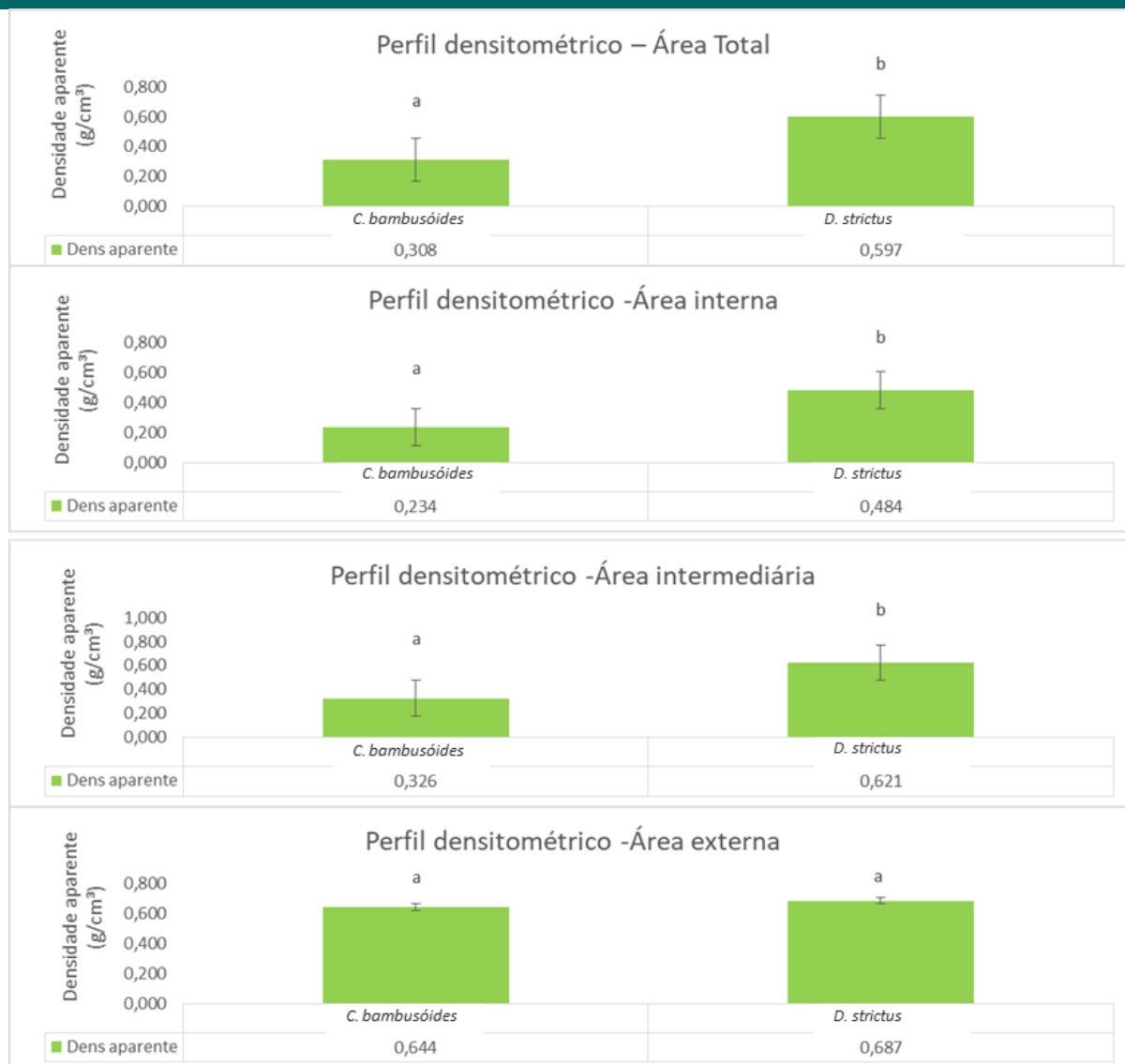
Figure 6 – Comparison of the transverse densitometric profile of Chusquea bambusoides and Dendrocalamus strictus samples across the three transverse areas of their culms (inner, intermediate and outer) and across the entire transverse area.
