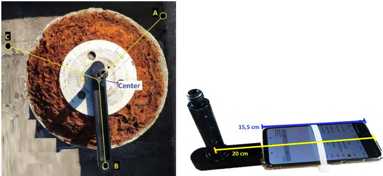
**Figure 1:** On the left, the figure shows the position of the support on the pillar oriented in relation to the point B. On the right, the figure shows the position of the smartphone to the support and its dimensions.
