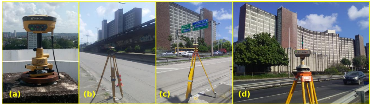
Figure 2: (a) GNSS Topcon Hiper V receiver at SAT GPS station 91551; (b), (c) and (d) GNSS Topcon Hiper Lite + receivers measuring the immediate support points (P1, P2 and P3 respectively) near the building.
