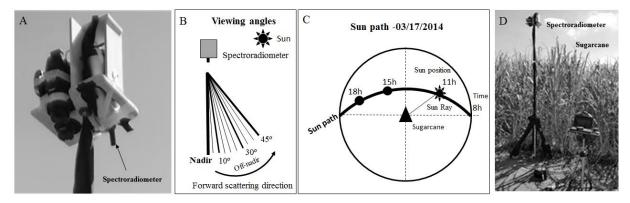
Figure 2: A) Sensors installed in the holder. B) Forward scattering direction. C) Sun path diagram 03/17/2014. D) Sensor support on canopy of sugarcane.
