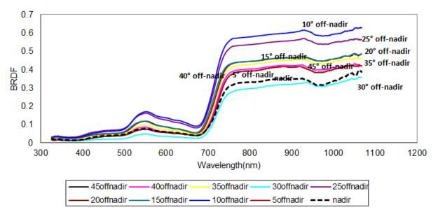
**Figure 3:** Bidirectional Reflectance Distribution Function of sugarcane, measured at different viewing angles.
