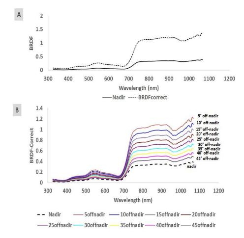
**Figure 6:** (A) Comparison between spectral reflectance profile with and without application of Walthall's BRDF correction model. (B) Spectral reflectance profile at different viewing angles applied to Walthall's BRDF correction model.
