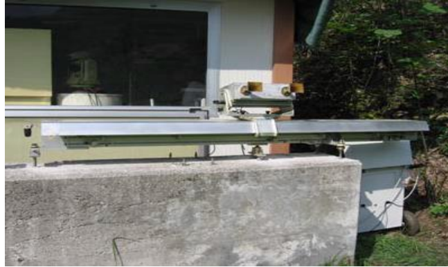
Figure 1: Micro-deformation monitoring system IBIS.
