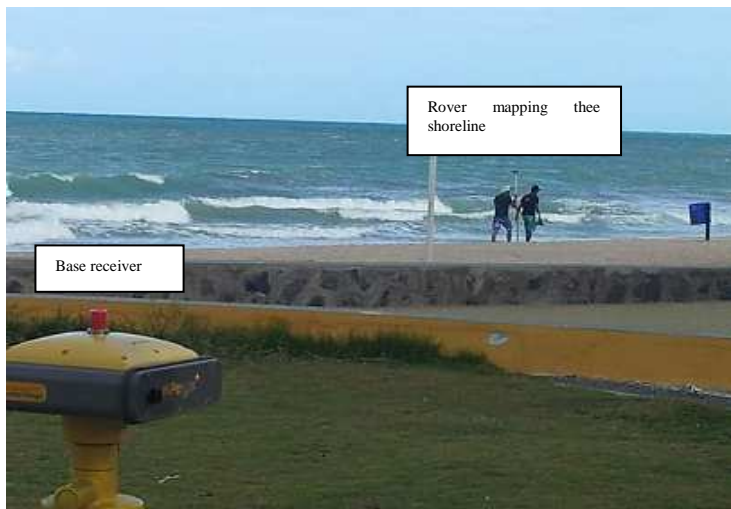
Figure 3 - Base and rover receiver in the study area.
